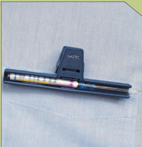
^ Figure 3 Note the end of the color change and record your reading. Then, simply divide by the number of hours for the TWA (PPM hours/hours worked).
